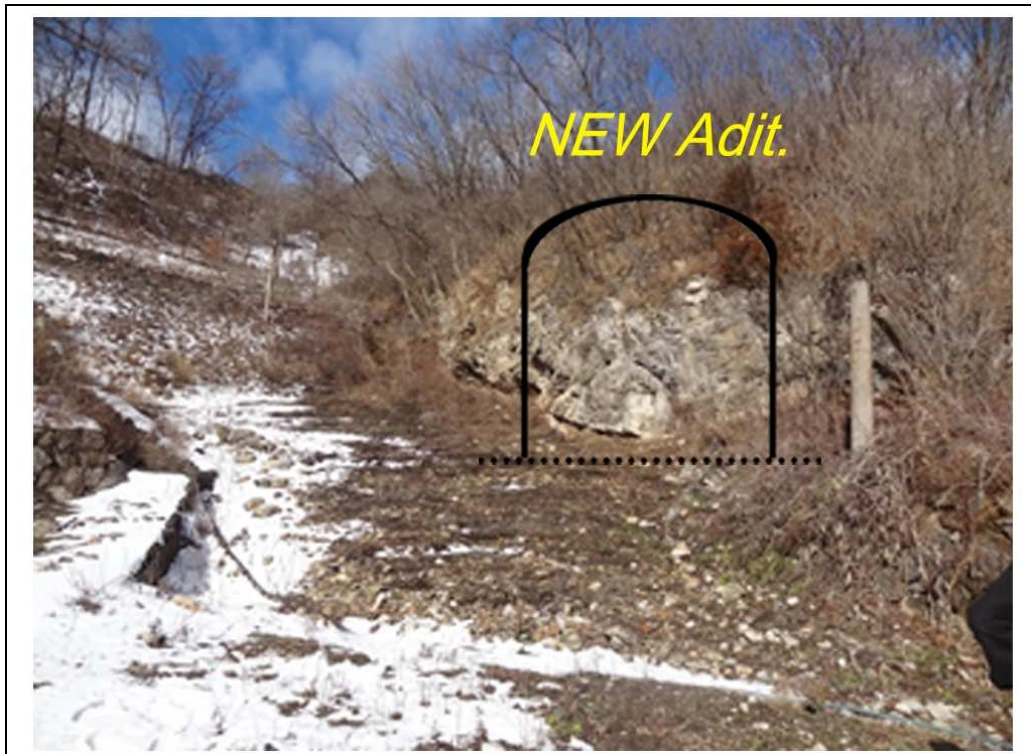
Figure 16-33. New Adit Portal Position, For -1 Level
